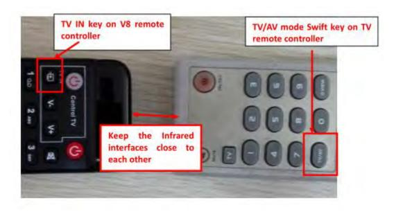
Note: During copying period, please keep the two remote controllers Infrared interfaces close to each other. If it fails to copy, you can try once again. However, we cant make sure all remotes can copy successfully.
