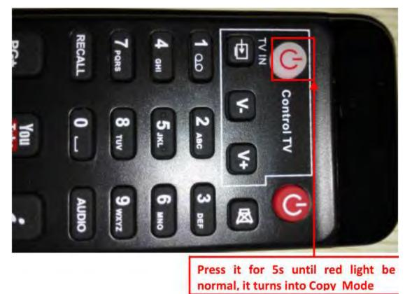
For example: Learn how to swift TV IN mode (There are four keys on V8 series remote controller in Control TV area and all of them can do copy).
